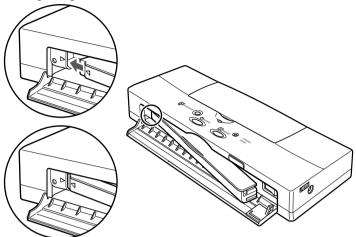
**4.** Push in on the right side of the battery pack to lock it in place.
